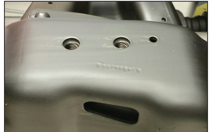
Upfit Body Frame ZW9 Attachment Provisions Figure 21
