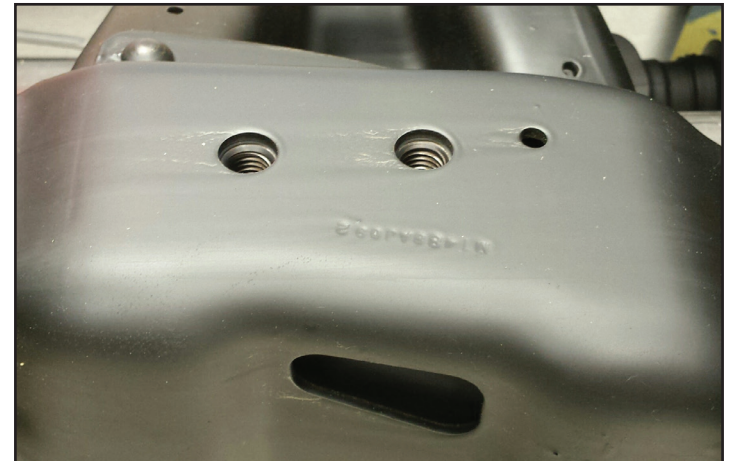
Upfit Body Frame ZW9 Attachment Provisions Figure 21
