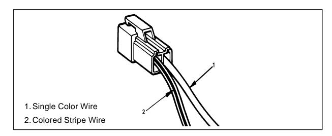
Abbreviations are used to indicate wire color within a circuit diagram. Refer to the following table
