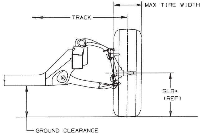
\* MINIMUM GROUND CLEARANCE TO BE CALCULATED BY USING GROSS AXLE HEIGHT AND RECOMMENDED TIRE PRESSURE
