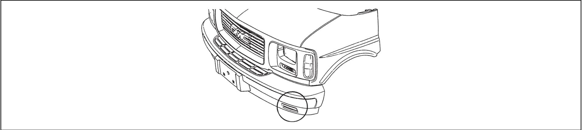
All G10 and some G20 models are equipped with front air dams below the front bumper as shown in the illustration. These air dams are equipped with brake cooling openings as shown. These openings should not be obstructed by the addition of any accessories that would impede the flow of air to the front brakes.
