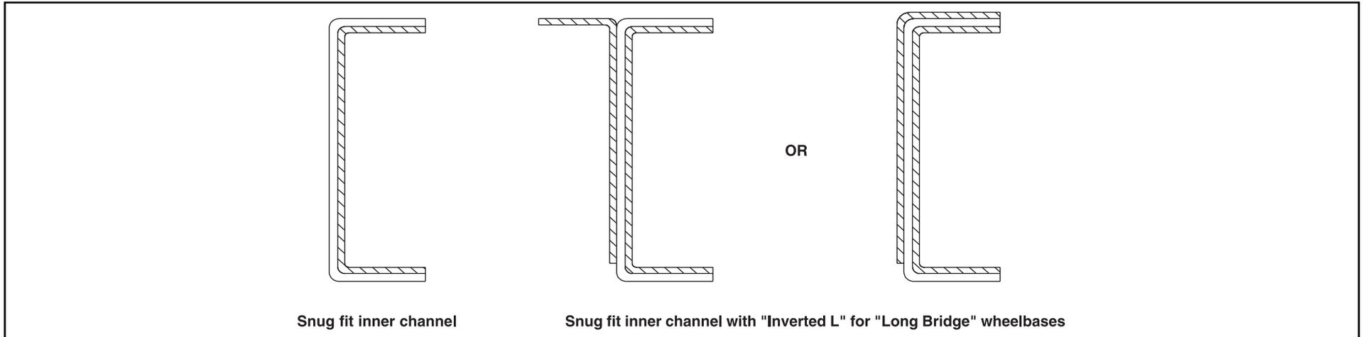
7. The reinforcements must be fastened securely to only the web of the original chassis frame rail. The reinforcement must be held rigidly in place using either HUC bolts, GRADE 8 bolts and hardened steel washers at both the bolt head and nut, or GRADE 8 flanged bolts and hardened steel washers at the nut. Below are some suggested bolt patterns. It should be noted that these bolt patterns must not align the bolts vertically, i.e.: the bolt pattern must be staggered.
