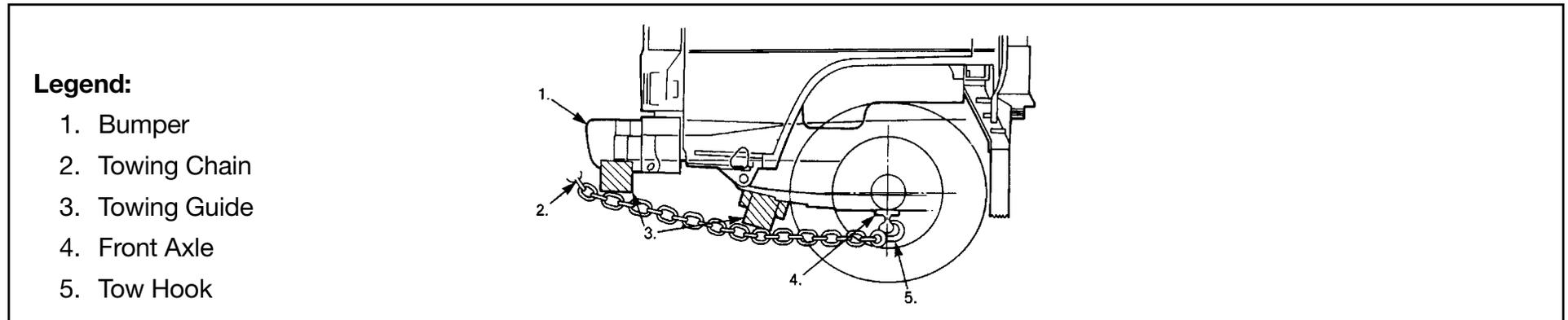
To prepare a disabled vehicle for front end towing with all wheels on the ground, the following steps are necessary:
