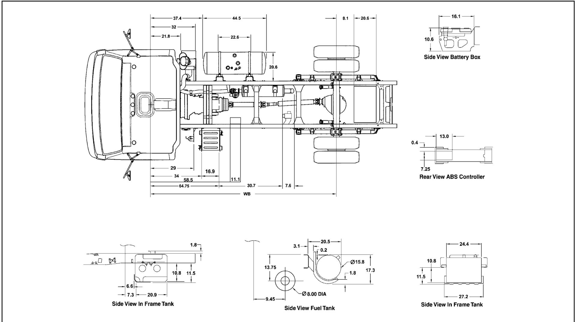
**NOTE:** Frame-mounted fuel tank available on 109", 132.5", 150" and 176" WB as an option replacing the In-Frame Tank.
