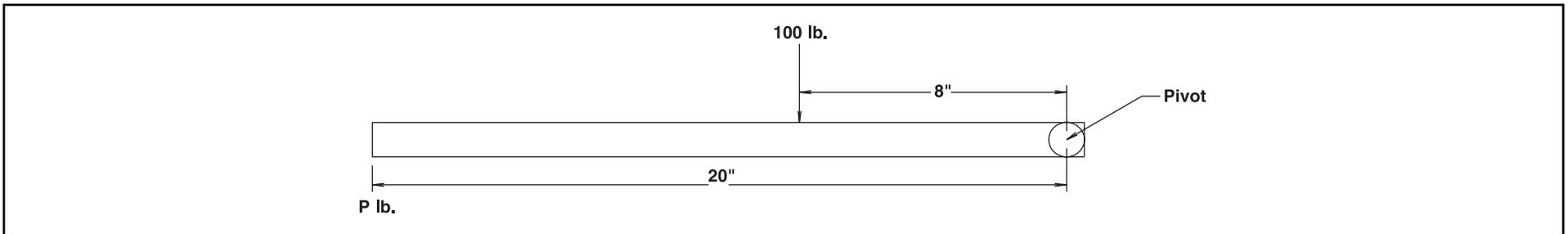
To find the value of “P”, the leverages must be equal for balance.
