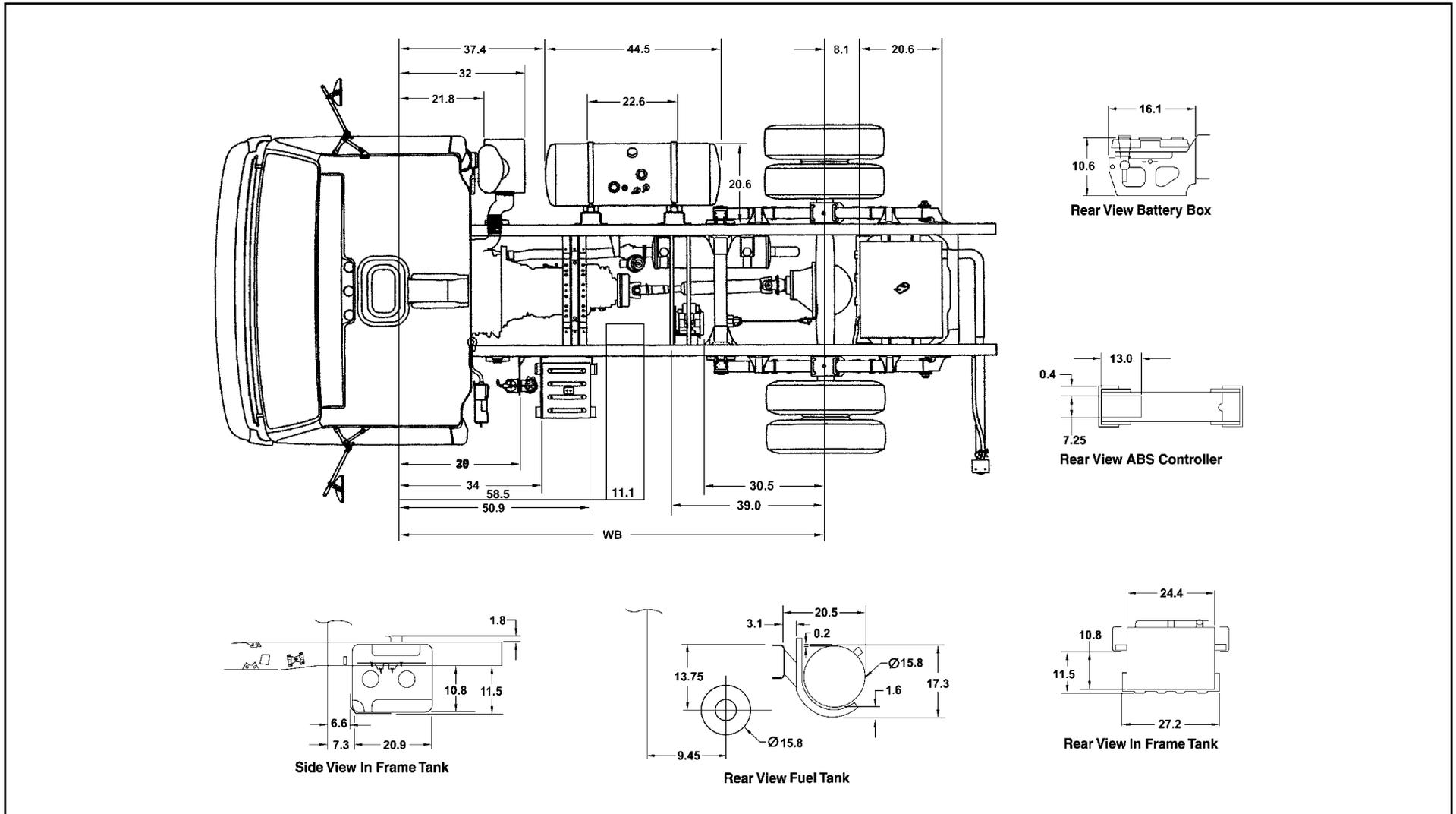
**NOTE:** Frame-mounted fuel tank available on 109", 132.5", 150" and 176" WB as an option. Allow 3" additional for battery box opening clearance.
