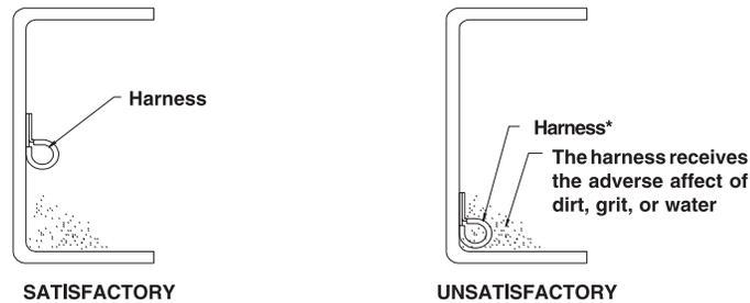
\* Harnesses should not be installed on inside lower face of the chassis frame.
