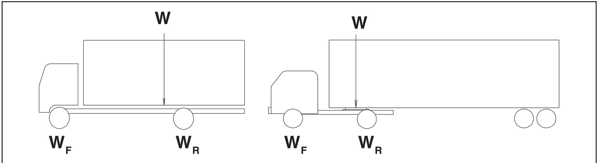
The weight at the center of the body and the load when applied is the same as the single point load of the kingpin on the fifth wheel.
