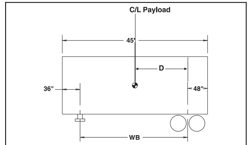
In the following example, a 50,000-pound payload at water-level loading. Calculate the payload (PL) weight transfer to kingpin and the rear axle.
