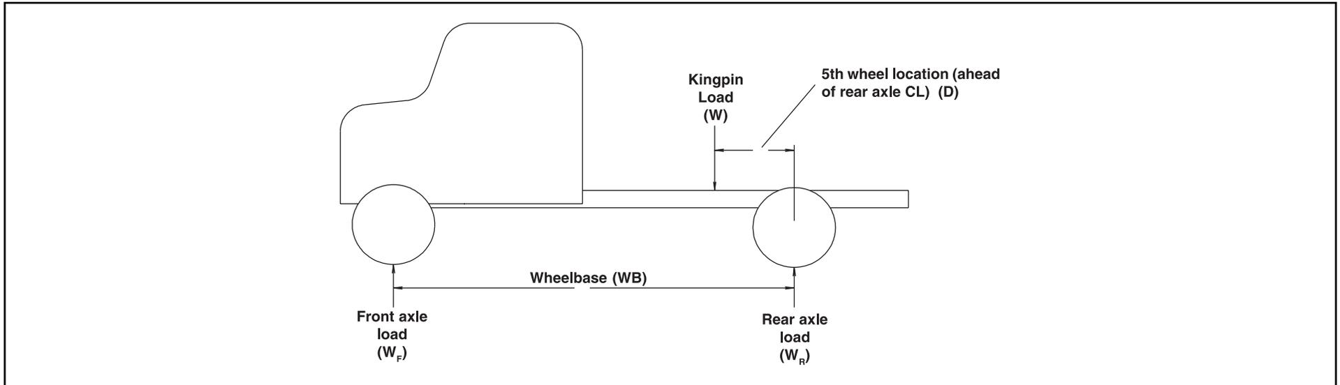
$$\text{Front Axle Load:} = \frac{\text{Kingpin Load} \times \text{5th Wheel Location}}{\text{Wheelbase}}$$
