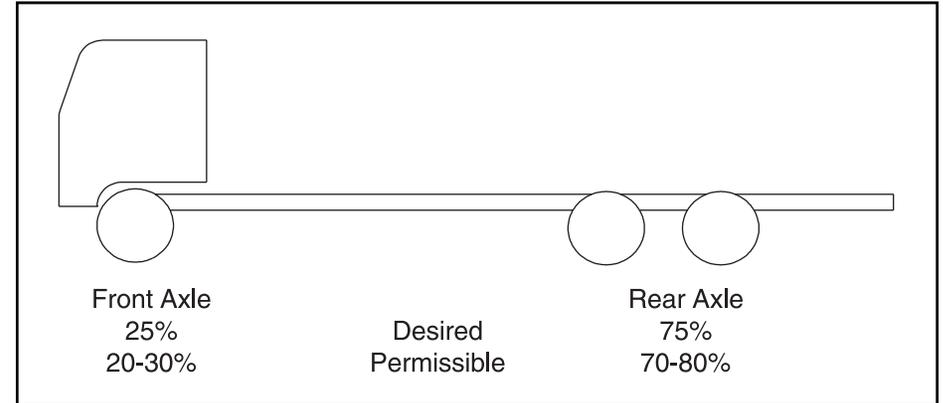
Calculating tractor/trailer weight distribution can be thought of in the same terms as calculating full trucks.
