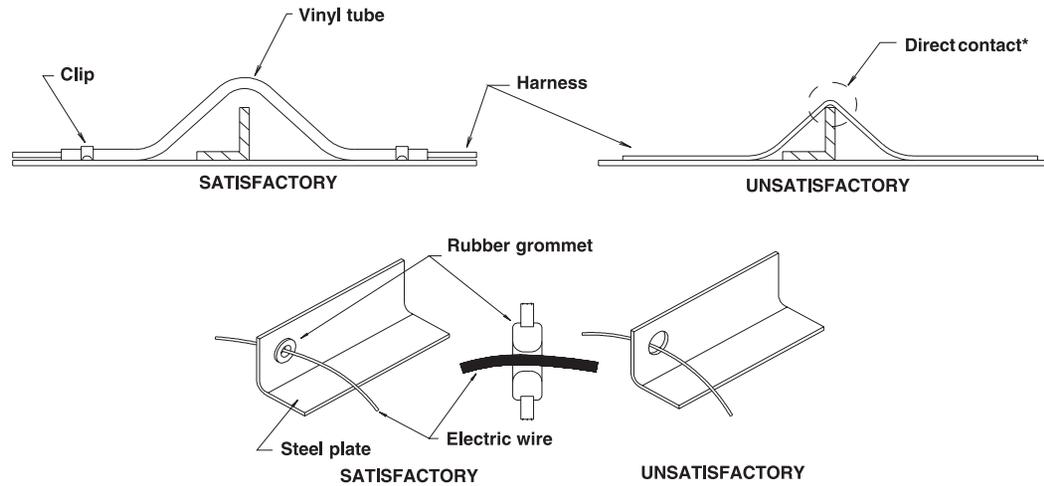
\* Cables should not be in contact with sharp edges or pierced holes.
