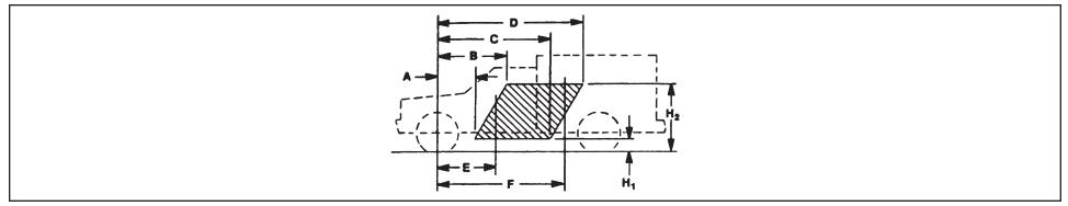
C/G of vehicle in CMVSS or FMVSS unladen condition [Curb + 181.4 kg. (400 lb) or Curb + 226.8 kg. (500 lb) as defined by CMVSS 105 and FMVSS 105] must be inside shaded area - that is, the C/G must be within the trapezoid formed by the coordinates A, B, C, D, H<sub>1</sub>, & H<sub>2</sub>, plus the C/G must be to the rear of vertical line E and forward of vertical line F.
