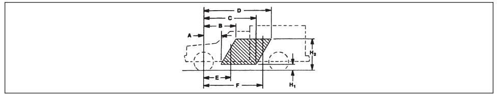
C/G of vehicle in CMVSS or FMVSS unladen condition [Curb + 181.4 kg. (400 lb)] must be inside shaded area – that is, the C/G must be within the trapezoid formed by the coordinates A, B, C, D, H<sub>1</sub>, & H<sub>2</sub>, plus the C/G must be to the rear of vertical line E and forward of vertical line F.
