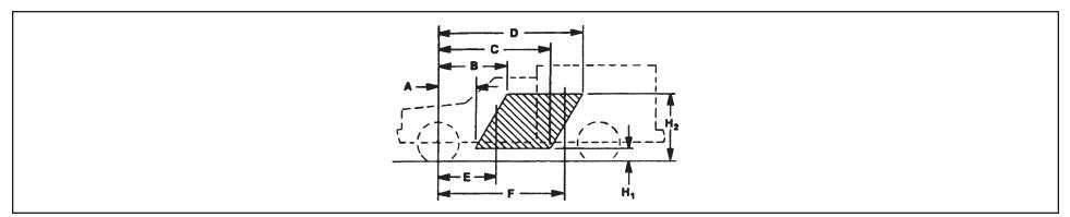
C/G of vehicle in CMVSS or FMVSS unladen condition [Curb + 181.4 kg. (400 lb) or Curb + 226.8 kg. (500 lb) as defined by CMVSS 105 and FMVSS 105] must be inside shaded area – that is, the C/G must be within the trapezoid formed by the coordinates A, B, C, D, H<sub>1</sub>, & H<sub>2</sub>, plus the C/G must be to the rear of vertical line E and forward of vertical line F.
