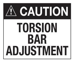
To help avoid personal injury, refer to Z-height setting procedure before adjusting torsion bars. If torsion bars are adjusted for aftermarket equipment, be sure to return them to specification when the equipment is removed. Otherwise, a front shock absorber may dislodge and damage a front brake line. This could result in an accident when minimum stopping distances are required.
