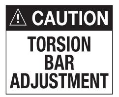
To help avoid personal injury, refer to Z-height setting procedure before adjusting torsion bars. If torsion bars are adjusted for aftermarket equipment, be sure to return them to specification when the equipment is removed. Otherwise, a front shock absorber may dislodge and damage a front brake line. This could result in an accident when minimum stopping distances are required.
