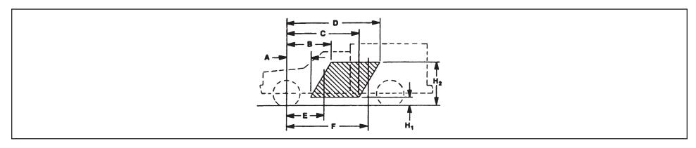
C/G of vehicle in CMVSS or FMVSS unladen condition [Curb + 181.4 kg. (400 lb)] must be inside shaded area – that is, the C/G must be within the trapezoid formed by the coordinates A, B, C, D, H<sub>1</sub>, & H<sub>2</sub>, plus the C/G must be to the rear of vertical line E and forward of vertical line F.
