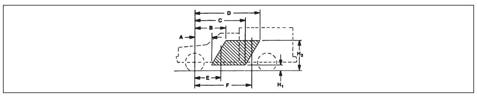
C/G of vehicle in CMVSS or FMVSS unladen condition [Curb + 181.4 kg. (400 lb)] must be inside shaded area – that is, the C/G must be within the trapezoid formed by the coordinates A, B, C, D, H<sub>1</sub>, & H<sub>2</sub>, plus the C/G must be to the rear of vertical line E and forward of vertical line F.
