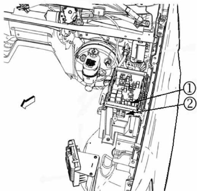
**Important:** A J-case fuse (1) with a 40 amp maximum rating MUST be inserted into this position (1) for the stud (2) to be powered.
