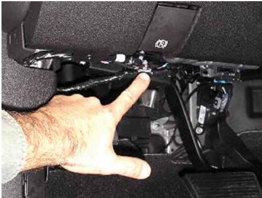
1. Locate the trailer brake control circuits that are looped and taped to the main harness under the instrument panel.
