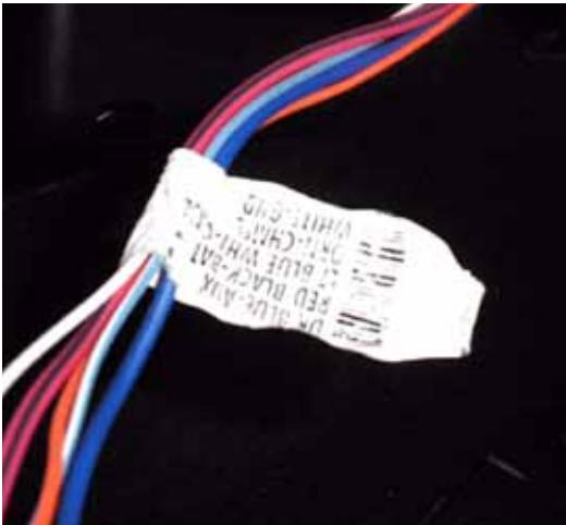
3. Match the vehicle harness label circuit functions to the trailer brake controller jumper harness functions.
