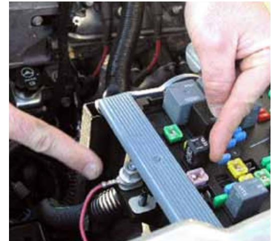
**Important:** Ensure that the ringlets are not interfering with the UBEC cover.
