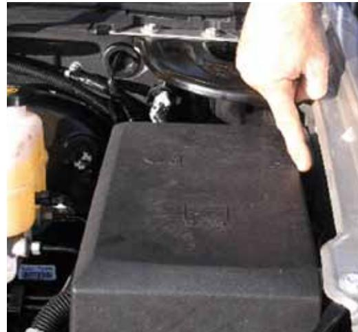
4. After completing the under dash connections to the electric brake controller, open the hood and locate the red wire that is taped to the harness between the underhood electrical center and the driver side front fender.
