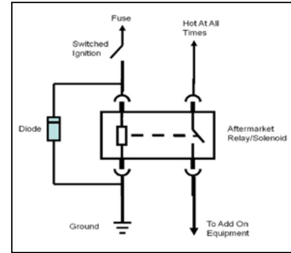
Install a diode, P/N 12112422, across the coil of the solenoid. It is important that the striped end of the diode be connected to the positive terminal of the coil and the other end of the diode be connected to ground.
