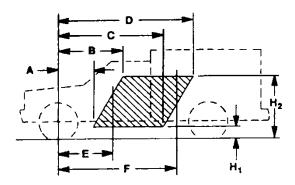
C/G of vehicle in CMVSS or FMVSS unladen condition [Curb + 181.4 kg. (400 lb) or Curb + 226.8 kg. (500 lb) as defined by CMVSS 105 and FMVSS 105] must be inside shaded area – that is, the C/G must be within the trapezoid formed by the coordinates A, B, C, D, H1, & H2, plus the C/G must be to the rear of vertical line E and forward of vertical line F.
