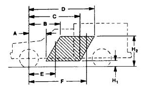
C/G of vehicle in CMVSS or FMVSS unladen condition [Curb + 181.4 kg. (400 lb)] must be inside shaded area – that is, the C/G must be within the trapezoid formed by the coordinates A, B, C, D, H1, & H2, plus the C/G must be to the rear of vertical line E and forward of vertical line F.
