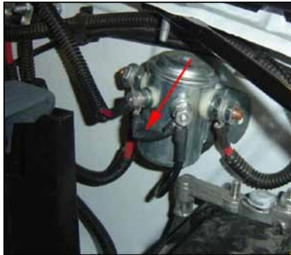
**Important:** Be sure to insulate the diode with heat shrink tubing before installing as shown in the picture above.
