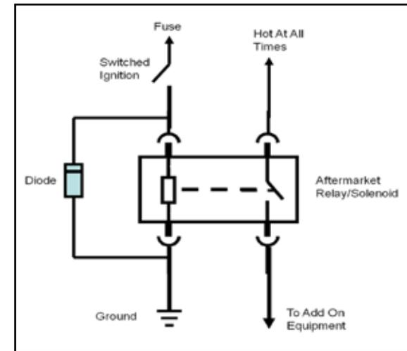
Install a diode, P/N 12112422, across the coil of the relay. It is important that the striped end of the diode be connected to the positive terminal of the coil and the other end of the diode be connected to ground. Be sure to insulate the diode with heat shrink tubing before installing.
