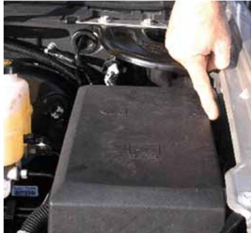
4. After completing the under dash connections to the electric brake controller, open the hood and locate the red wire that is taped to the harness between the underhood electrical center and the driver side front fender.
