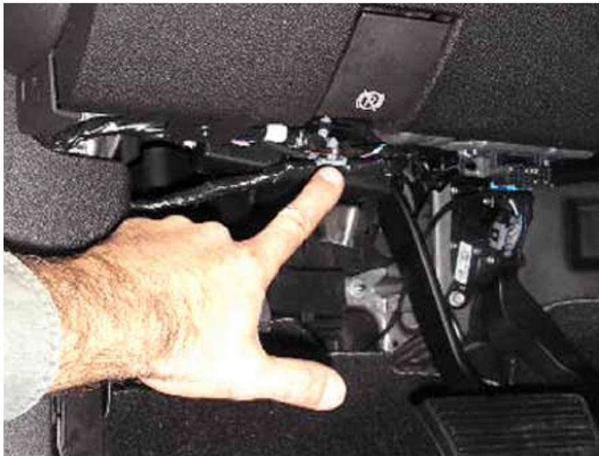
1. Locate the trailer brake control circuits that are looped and taped to the main harness under the instrument panel.
