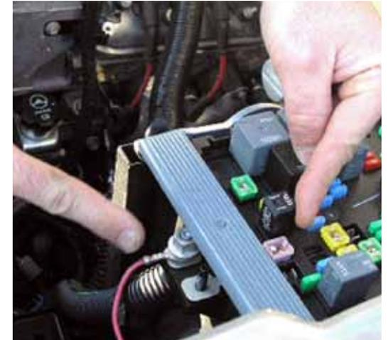
**Important:** Ensure that the ringlets are not interfering with the UBEC cover.
