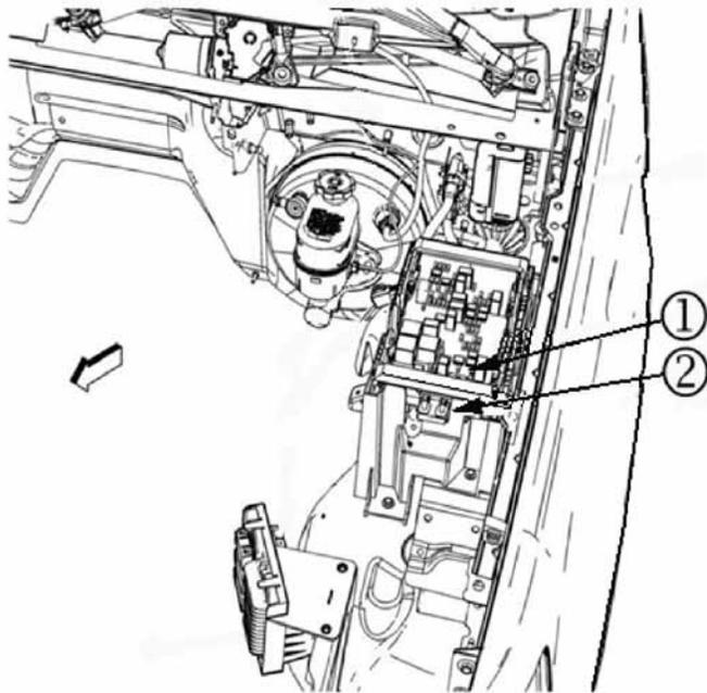
**Important:** A J-case fuse (1) with a 40 amp maximum rating **MUST** be inserted into this position (1) for the stud (2) to be powered.
