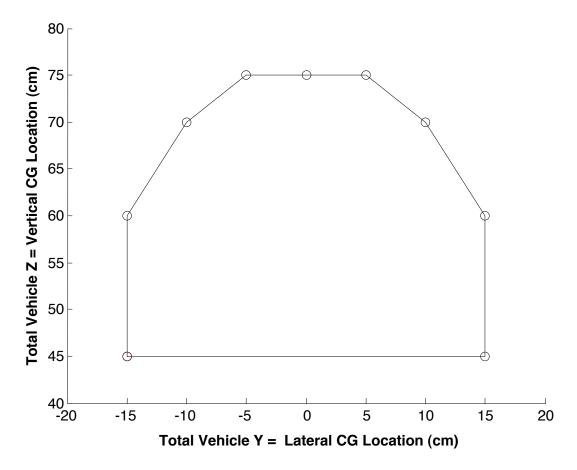
For Body Builder's use and applicable to CMVSS 126 and FMVSS 126, the longitudinal and vertical vehicle center of gravity location can be approximated by following the formula below and by referencing data elements within CMVSS 105 and FMVSS 105 – HYDRAULIC AND ELECTRIC BRAKE SYSTEMS or CMVSS 135 and FMVSS 135 LIGHT VEHICLE BRAKE SYSTEMS, ... ALLOWABLE CENTER OF GRAVITY CHARTS.
