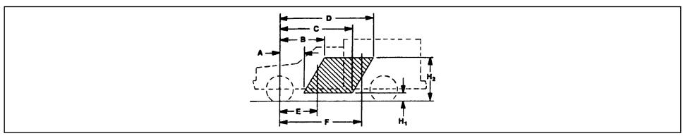
C/G of vehicle in CMVSS or FMVSS unladen condition [Curb + 181.4 kg. (400 lb) or Curb + 226.8 kg. (500 lb) as defined by CMVSS 105 and FMVSS 105] must be inside shaded area – that is, the C/G must be within the trapezoid formed by the coordinates A, B, C, D,  $H_1$ , &  $H_2$ , plus the C/G must be to the rear of vertical line E and forward of vertical line F.
