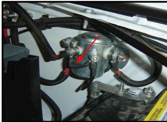
**Important: Be sure to insulate the diode with heat shrink tubing before installing as shown in the picture above.**
