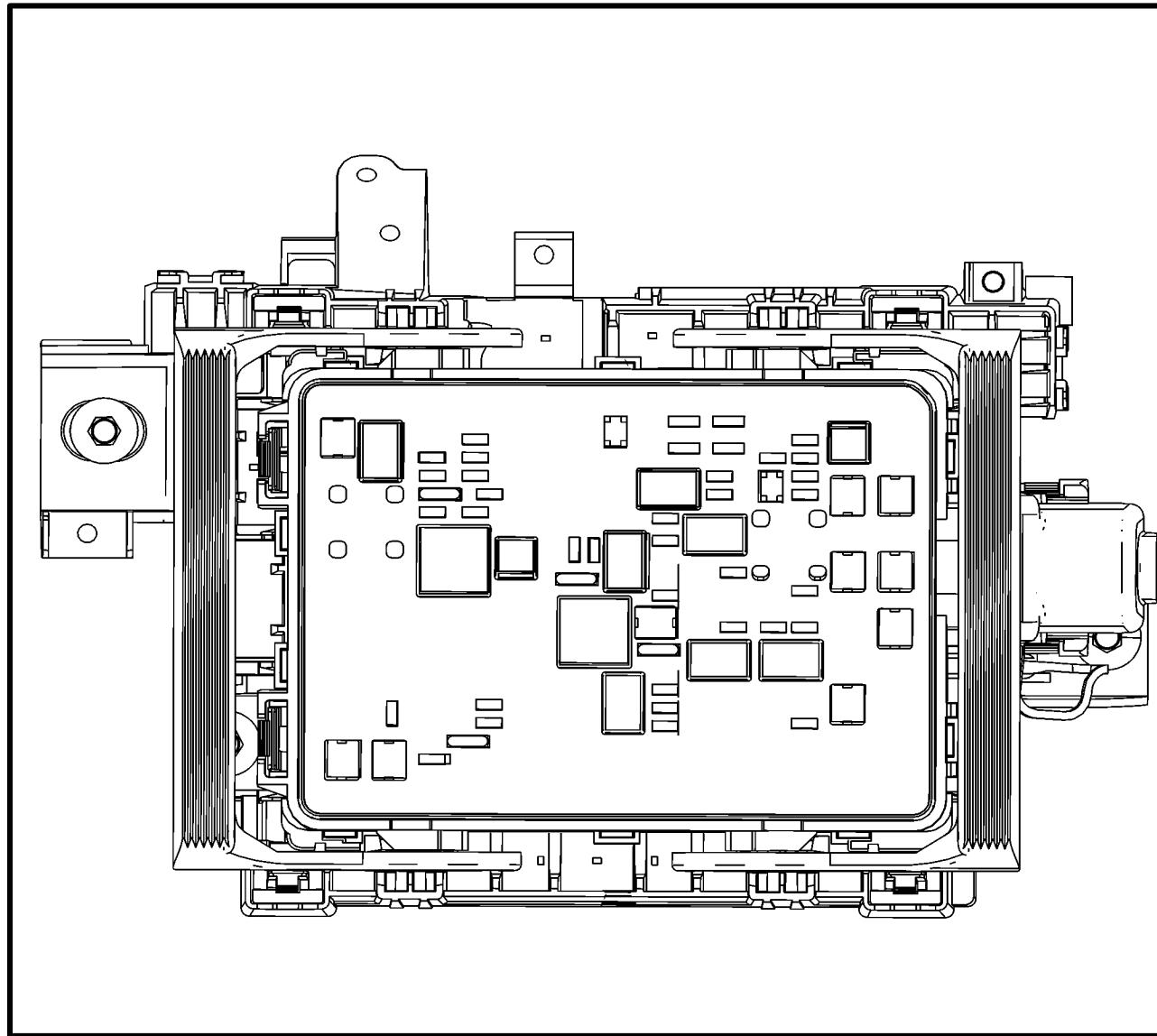
**Fuse Block (X50) Under-hood - Bottom View**
