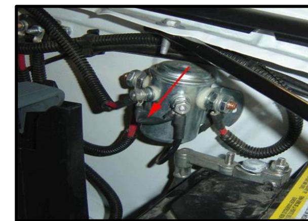
**Important: Be sure to insulate the diode with heat shrink tubing before installing as shown in the picture above.**
