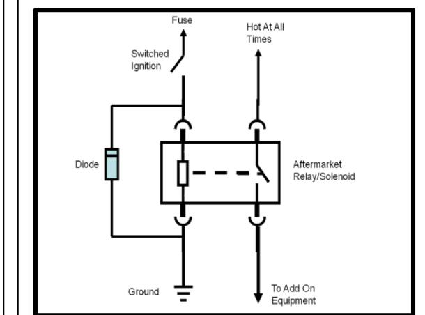
Install a diode, P/N 12112422, across the coil of the relay. It is important that the striped end of the diode be connected to the positive terminal of the coil and the other end of the diode be connected to ground. Be sure to insulate the diode with heat shrink tubing before installing.
