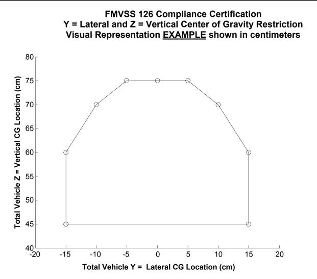
For Body Builder's use and applicable to CMVSS 126 and FMVSS 126, the longitudinal and vertical vehicle center of gravity location can be approximated by following the formula below and by referencing data elements within CMVSS 105 and FMVSS 105 – HYDRAULIC AND ELECTRIC BRAKE SYSTEMS or CMVSS 135 and FMVSS 135 LIGHT VEHICLE BRAKE SYSTEMS, ... ALLOWABLE CENTER OF GRAVITY CHARTS.
