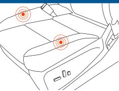
The Safety Alert Seat is part of the Lane Departure Warning (LDW) system and will provide three vibration pulses to the left seat side or right seat side, depending upon the side of the driving lane that the vehicle is moving toward. Also activated in reverse when objects are detected.
