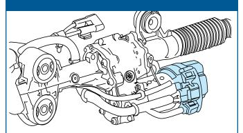
The Electric Power Steering System consists of a Rack-and-Pinion steering gear assisted by an electronically controlled power steering motor and drive assembly. The steering gear is mechanically connected to the steering wheel system.
