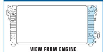
Engine Oil and Transmission Oil are cooled by passing the fluids through separate coolers located in the engine radiator assembly end tanks and the air conditioning condenser
