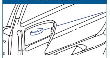
Rear door locking rods are disabled. Rear door locks are inoperable at rear doors, but operate from driver position. Inside rear door handles are disconnected. Rear doors can only be opened from the outside.
