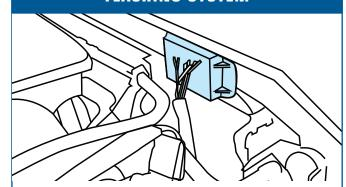
Option 6J7 provides a headlamps high beam flashing module, rear lamps flashing via the Body Control Module (BCM) and a control wire for customer-furnished switching to turn the module on and off. The flasher control wire is part of the blunt-cut upfitter harness coiled under the instrument panel in the front passenger side foot well. The flashing module is located on the rear edge of the right hand upper radiator support.
