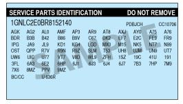
A Service Parts Identification (SPID) Label provides Vehicle Identification Number (VIN)-specific Option Code content list, Engineering Model Number (Nameplate, body style), Exterior paint system, Exterior paint color code and Interior trim level and color. The SPID label for the Tahoe is located on the inner surface of the instrument panel storage compartment (glove box).
