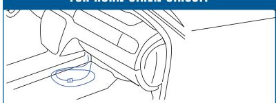
This provision permits customer connection of a switch to select either horn of siren operation when the horn pad is pressed.
