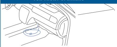
Approximately 60 inches (1.5 m) of auxiliary speaker wiring is routed from the front door and windshield pillar speakers and coiled under the instrument panel. The wiring permits connection of the front speaker pairs to customer-installed communication equipment. Vehicle radio front speaker outputs are re-routed to the rear speakers to maintain the required open door/key-in-ignition and other audible warnings. **NOTE: For wiring diagram see Wiring Section**
