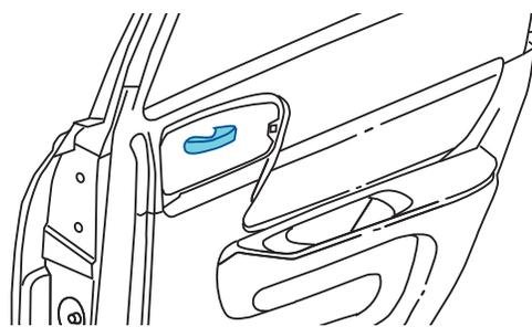
Rear doors can only be opened from the outside. Locks operate only from driver door switch
