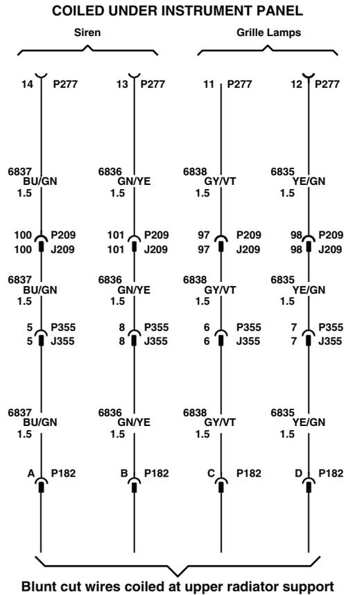
The SEO 6J3 wiring provision circuits are terminated in the 16 cavity connector at the front of the equipment mounting platform on the passenger side. The wiring circuits are routed from the passenger compartment to a 2 foot (30 cm) coil secured in the area behind the grille. There are four 16 gauge (1.5 mm) wires for connecting to the grille lights and siren speaker.
