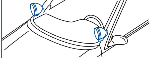
7X6 Spotlamp left hand, pillar-mounted unity, 6-inch with replaceable H3 halogen bulb; independently fused
