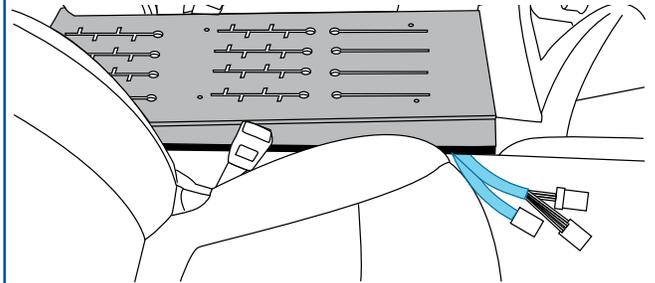
The SEO 6J3 wiring provision circuits are terminated at a 16-way connector on the upfitter harness at the front of the equipment mounting platform. The wiring circuits are routed from under the instrument panel to a 2-foot (610 mm) coil secured in the area behind the grille, to the left of the hood latch assembly.
