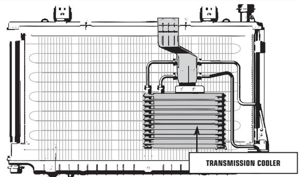
The transmission cooler is positioned to the left side, in front of the air conditioning condenser. The cooling system is common to the V6 and V8 engines
