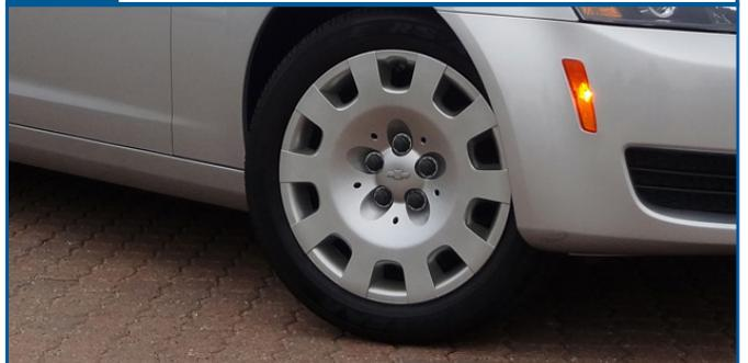
Plastic wheel cover attaches to threaded lug nuts
