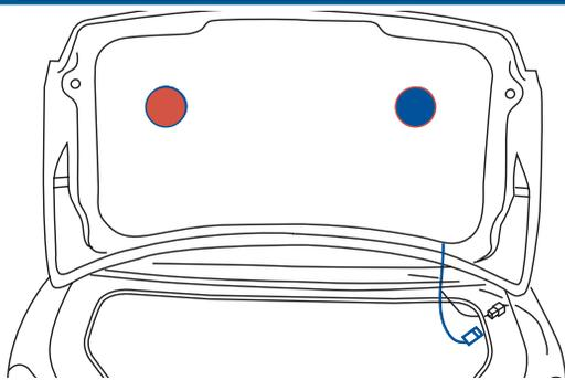
Two 4-inch, single faced, red and blue LED lamps are mounted to the deck lid inner panel. Lamps are activated by the deck lid ajar mechanical switch when deck lid is opened. Lamps are wired to flash alternately through a flasher located at the upper right hand corner of the trunk opening.
