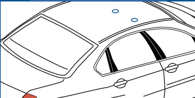
6B7 Hole is drilled near center line of roof panel approximately 29 inches rearward of windshield opening. Includes sealing harness grommet in roof hole
