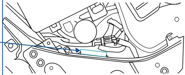
Option 6J7 provides a headlamps high beam flashing module, rear lamps flashing via the Body Control Module (BCM) and a control wire for customer-furnished switching to turn the module on and off. The flasher control wire is terminated in the 16-way connector on the upfitter harness at the right front corner of the equipment mounting platform. The flashing module is located on the rear side of the passenger side upper radiator support
