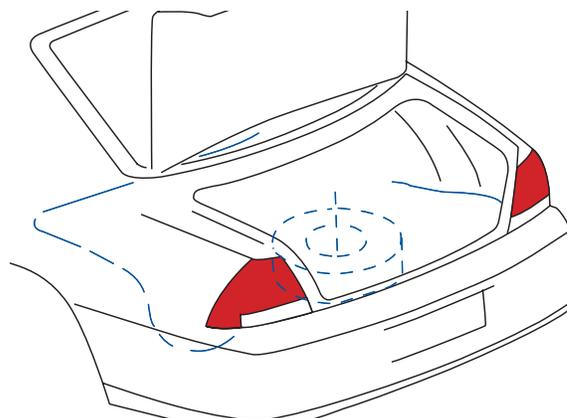
Full-size spare tire is mounted under the load floor. The full-size spare tire includes a Tire Pressure Monitor (TPM) sensor which must be programmed to the TPM System after the spare tire is installed.
