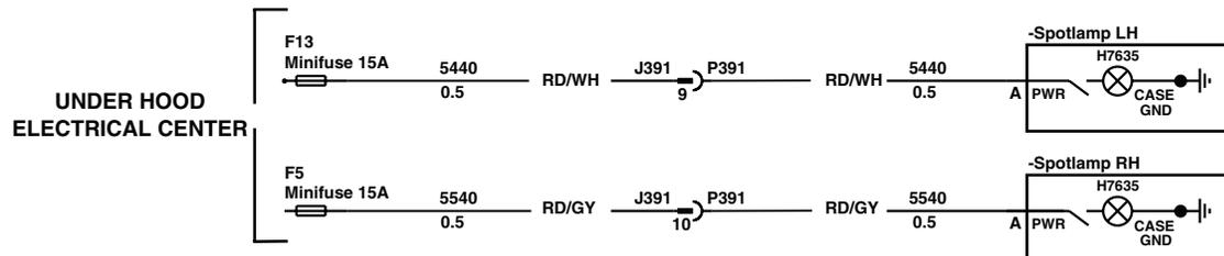
7X6 spotlamp left hand and 7X7, spotlamps left and right hand, pillar-mounted Unity, 6-inch with replaceable H3 halogen bulb; independently fused
