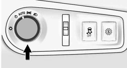
**VVS** – Delete Daytime Running Lamps and Automatic Headlamps. This option disables the Daytime Running Lamps and Automatic Headlamps control feature. Exterior lamps are manually controlled only. Option VVS is not available in Canada. The headlamp control on the driver's side of the instrument panel operates the headlamps.
