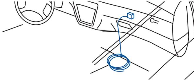
Two 16-gauge wires are connected to an in-line connector in the horn circuit of the instrument panel harness under the instrument panel. The end of this harness extension is terminated with an in-line connector in a 60-inch (1.5 m) coil under the instrument panel. Connection to customer switching permits operation of the horn or siren with the horn button.
