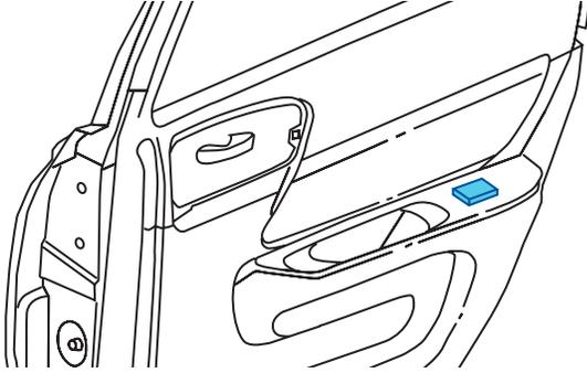
Rear door window switches are inoperable. Rear door power regulators are operable only from driver position switches.
