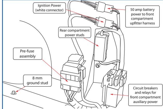
An auxiliary power junction block is located at the right side of the trunk. The junction block is at the rear of the auxiliary battery tray and contains a split buss with two terminals for customer connection to 12-volt battery power.
