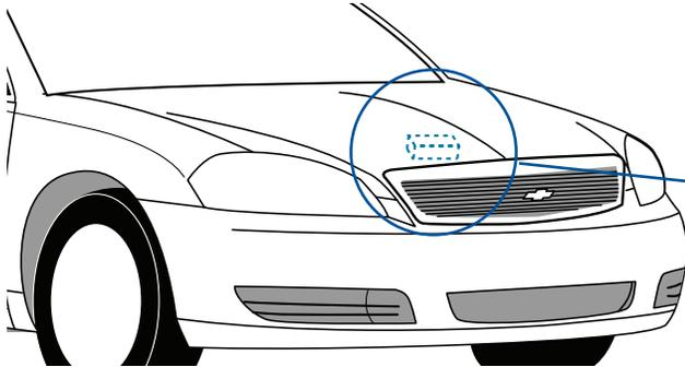
The Option 6J7 Exterior Lamps Emergency Flashing Module mounting location at the rear edge of the upper right hand radiator support.
