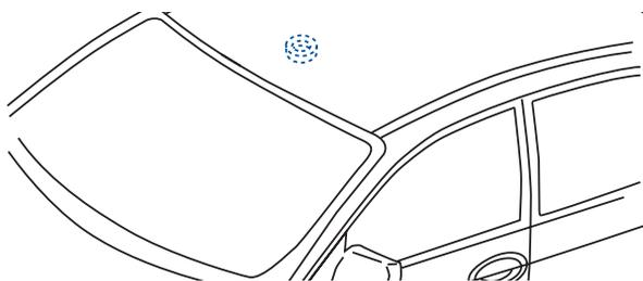
Red and white auxiliary dome lamp is located to the rear of the vehicle dome lamp (red is LED and white is incandescent). The auxiliary lamp is wired independently from the standard dome lamp.
