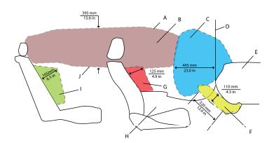
FRONT PASSENGER AND KNEE, DRIVER SEAT BACK SIDE, LEFT REAR SEAT BACK AND ROOF RAIL AIRBAGS
