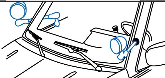
7X6 Spotlamp left hand, pillar-mounted unity, 6-inch with replaceable H3 halogen bulb; independently fused
