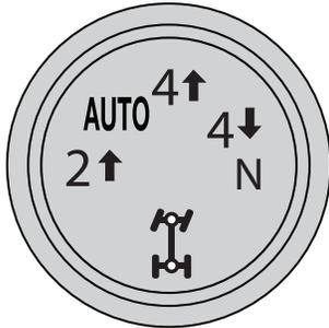
Active, 2-speed electronic Autotrac with rotary controls, includes neutral position for dingy towing. Use the transfer case knob next to the steering wheel to shift into and out of four-wheel drive.
