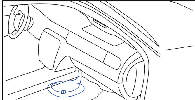
This provision permits customer connection of a switch to select either horn of siren operation when the horn pad is pressed.
