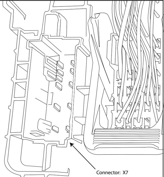
Connection to the circuits located in ICEM X7 must be made by a customer-provided jumper harness consisting of a connector and appropriately sized wires. The mating connector for ICEM cavity X7 is GM service part 19328970 (OEM 19324036). Refer to the wiring diagrams in this Specification for more information and to GM Upfitter Bulletin 115. A complete harness for connection to ICEM X7 is available from the GM police vehicle Second Stage Manufacturer, Kerr Industries (905 725 6561).
