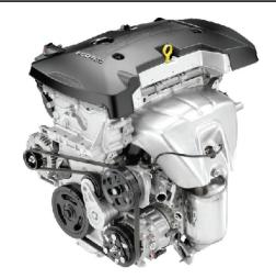
4-cylinder combines Direct Injection, Variable Valve Timing and stop/ start technology to help save on gas. Stop/start technology can automatically shut off the engine when stopped and enables a smooth transition when the brake pedal is released.
