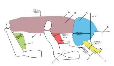
FRONT OUTBOARD PASSENGER FRONTAL AIRBAG AND KNEE AIRBAG, DRIVER AND LEFT REAR SEAT BACK SIDE IMPACT AIRBAGS AND LEFT ROOF RAIL MOUNTED HEAD-CURTAIN AIRBAG.
