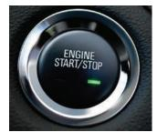
**STARTING THE ENGINE.** With the vehicle in Park or Neutral, press the brake pedal and then press and hold the ENGINE START/STOP button to start the engine.
