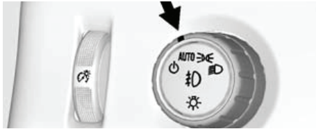
Exterior Lamp Controls here
