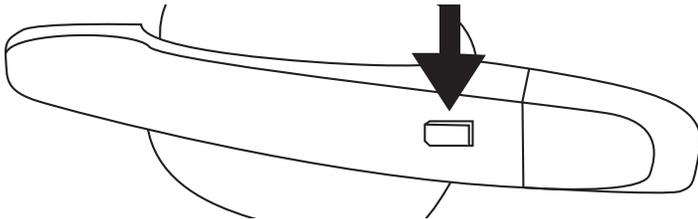
When the doors are locked and the RKE transmitter is within 3 ft (1 m) of the driver door handle, pressing the lock/unlock button on the driver door handle will unlock the driver door. If the lock/unlock button is pressed again within five seconds, all passenger doors will unlock. Pull the door handle to unlatch the door. Pressing the lock/unlock button will cause all doors to lock if any of the following occur.
