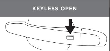
When the doors are locked and the RKE transmitter is within 3 ft (1 m) of the driver door handle, pressing the lock/unlock button on the driver door handle will unlock the driver door. If the lock/unlock button is pressed again within five seconds, all passenger doors will unlock. Pull the door handle to unlatch the door. Pressing the lock/unlock button will cause all doors to lock if any of the following occur.
