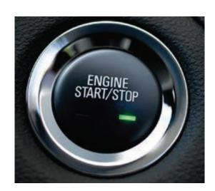
**STARTING THE ENGINE.** With the vehicle in Park or Neutral, press the brake pedal and then press and hold the ENGINE START/STOP button to start the engine.
