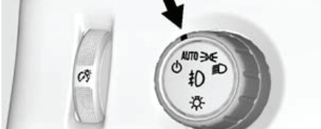
Exterior Lamp Controls here
