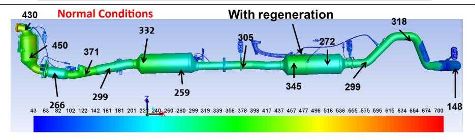
Note: These are typical exhaust skin and gas temperatures and the actual temperatures may vary based on specific operating and environmental conditions, as well as the specific body applications.
