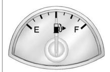
When the ignition is on, the fuel gauge shows how much fuel is left in the fuel tank. When the indicator nears empty, a message in the Driver Information Center (DIC) displays. See *Fuel System Messages on page 5-25*. The vehicle still has a little fuel left, but the vehicle should be fueled soon. An arrow on the fuel gauge indicates the side of the vehicle the fuel door is on.
