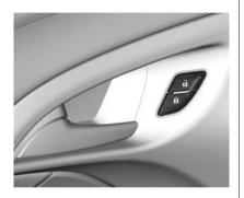
(Unlock): Press to unlock the doors.
