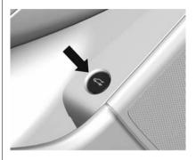
From inside the vehicle, press on the driver or passenger door. The ignition must be in ON/RUN or ACC/ACCESSORY, or the vehicle speed must be less than 3 km/h (2 mph) for the trunk release to operate.
