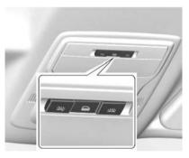
The dome lamp controls are on the front overhead console.
