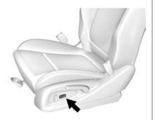
Press and hold the front or rear of the control to increase or decrease lumbar support. Release the control when the seatback reaches the desired level of lumbar support.
