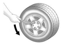
Turn the wheel wrench counterclockwise to loosen all the wheel nuts.
