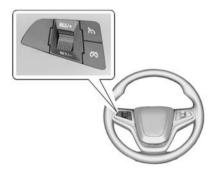
(On/Off): Press to turn the cruise control system on and off. A white indicator comes on in the instrument cluster when cruise is turned on.
