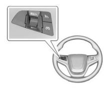
እ: Press to turn the cruise control system on and off. A white indicator comes on in the instrument cluster when cruise is turned on.
