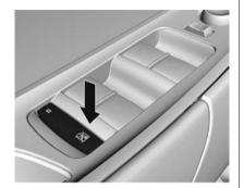
Press to prevent rear seat passengers from operating the windows. The indicator light illuminates when on. Press again to turn the feature off
