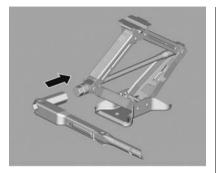
6. Slide the wheel wrench onto the drive nut of the jack.
