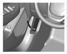
Pull up on the hood release handle with this symbol on it. It is located below the instrument panel to the left of the steering column.
