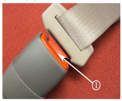
In the next photo, a 2010 buckle is substituted and a 2011 latch is inserted. When connected, the latch will not retain as closely to the housing, and a gap (1) will be visible.
