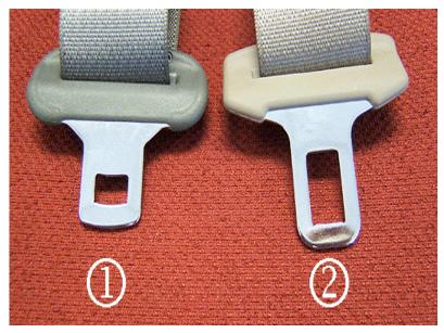
The buckle side of the seat belt also features a slightly revised appearance. The 2010 system has a buckle housing (1) that protrudes further from the plastic sleeve compared to the shorter 2011 housing (2). A smoother texturing is also used on the 2011 buckle, which differs from that of the sleeve.
