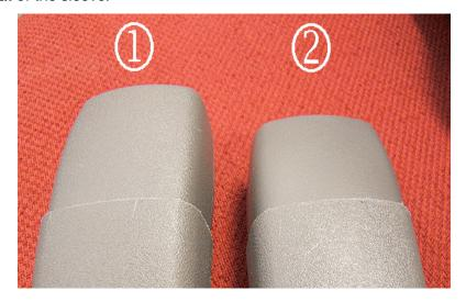
**Important:** The buckle side belt sleeve is not changed from 2010 to 2011 model vehicles. Another way of assuring both latch and buckle side components are of the same model year is to attempt to connect them.
