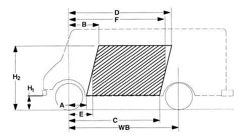
C/G of vehicle in CMVSS or FMVSS unladen condition [Curb + 181.4 kg. (400 lb) for vehicles less than or equal to 4536 kg (10,000 lbs) GVWR or Curb + 226.8 kg (500 lbs) for vehicles greater than 4536 kg (10,000 lbs) GVWR] must be inside shaded area – that is, the C/G must be within the trapezoid formed by the coordinates A, B, C, D, H1, & H2, plus the C/G must be to the rear of vertical line E and forward of vertical line F.
