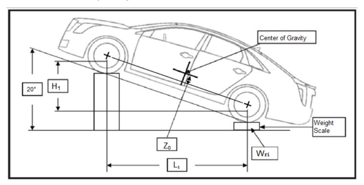
3. The **vertical** center of gravity location Z<sub>0</sub> is determined by:
