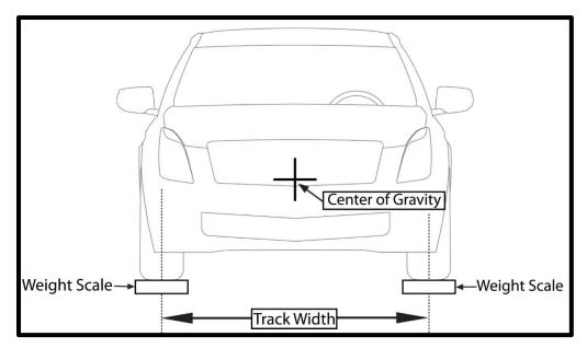
3. For all types of incomplete vehicles contained in this document with an average front track of 1587 mm (62.47 in), the **lateral** center of gravity location is determined by:
