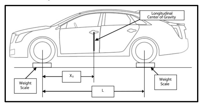
3. The **longitudinal** center of gravity location, X<sub>0</sub>, is determined by:
