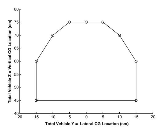
For upfitter use and applicable to CMVSS 126 and FMVSS 126, the longitudinal and vertical vehicle center of gravity location can be approximated by following the formula below and by referencing data elements within CMVSS 105 and FMVSS 105 – HYDRAULIC AND ELECTRIC BRAKE SYSTEMS or CMVSS 135 and FMVSS 135 LIGHT VEHICLE BRAKE SYSTEMS, ... ALLOWABLE CENTER OF GRAVITY CHARTS.
