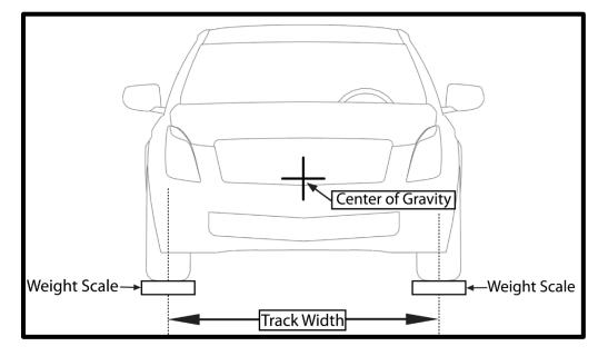
3. For all types of incomplete vehicles contained in this document with an average front track of 1587 mm (62.47 in), the **lateral** center of gravity location is determined by:
