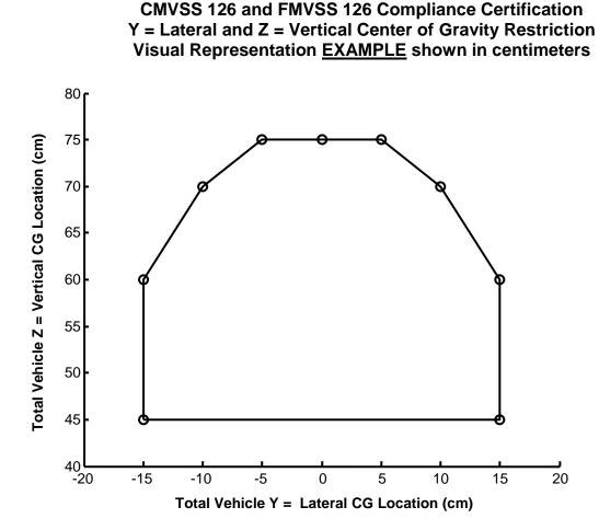
For upfitter use and applicable to CMVSS 126 and FMVSS 126, the longitudinal and vertical vehicle center of gravity location can be approximated by following the formula below and by referencing data elements within CMVSS 105 and FMVSS 105 – HYDRAULIC AND ELECTRIC BRAKE SYSTEMS or CMVSS 135 and FMVSS 135 LIGHT VEHICLE BRAKE SYSTEMS, ... ALLOWABLE CENTER OF GRAVITY CHARTS.
