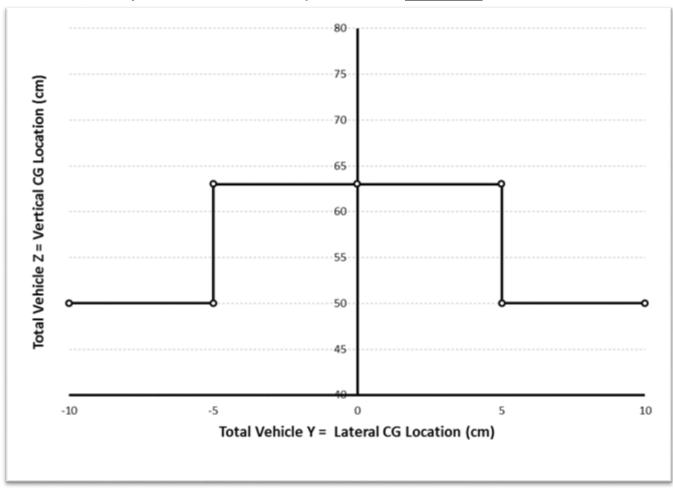
For upfitter use and applicable to CMVSS 126 and FMVSS 126, the longitudinal and vertical vehicle center of gravity location can be approximated by following the formula below and by referencing data elements within CMVSS 105 and FMVSS 105 – HYDRAULIC AND ELECTRIC BRAKE SYSTEMS or CMVSS 135 and FMVSS 135 LIGHT VEHICLE BRAKE SYSTEMS, ... ALLOWABLE CENTER OF GRAVITY CHARTS.
