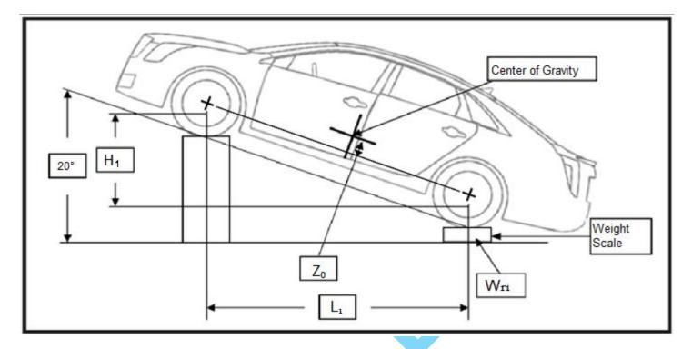
3. The vertical center of gravity location Z<sub>0</sub> is determined by:
