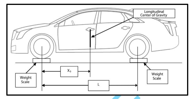
3. The longitudinal center of gravity location, X<sub>0</sub>, is determined by:
