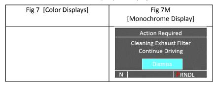
No stationary regen options remain at this time. If soot levels are allowed to go higher than 140% soot level a check engine light will be displayed and the engine will go into reduced power. At this point only a dealer can clean the DPF and restore normal operation. The DPF will clean itself if the vehicle can be driven
