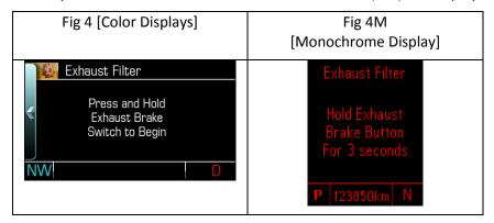
Hold the Exhaust Brake switch on the instrument panel [below the climate controls] for more than three seconds, and then release it, to begin the regeneration process. If the EXHAUST BRAKE ON message displays, then the switch was released too soon. Press it again to turn off the exhaust brake, then try again when the DIC message prompts.
