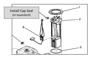
17. Cap the fuel inlet port which the fuel line from the rear tank was connected with a suitable cap and clamp.
