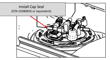
17. Install a cap seal on the fuel inlet port from rear tank.
