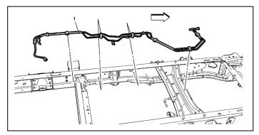
10. Disconnect the quick connect fittings and remove the fuel lines from the rear fuel tank to front/side fuel tank.
