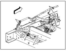
4. Disconnect the sending unit electrical connector
