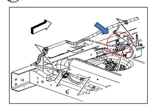
14. Disconnect the pressure balance pump electrical connector
