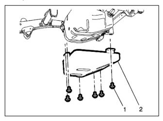
4. Remove the fuel tank shield bolts (1) and the fuel tank shield (2).
