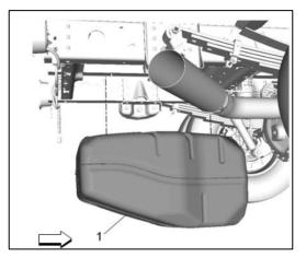
15. Remove Auxiliary Fuel Tank(1)
