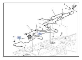
16. Remove the lines (15 & 20) from the rear tank to the front tanks.
