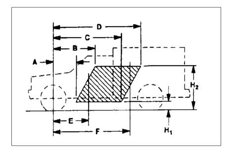
C/G of vehicle in CMVSS or FMVSS unladen condition [Curb + 181.4 kg. (400 lb) or Curb + 226.8 kg. (500 lb) as defined by CMVSS 105 and FMVSS 105] must be inside shaded area – that is, the C/G must be within the trapezoid formed by the coordinates A, B, C, D, H1, & H2, plus the C/G must be to the rear of vertical line E and forward of vertical line F.
