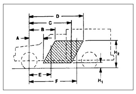
C/G of vehicle in CMVSS or FMVSS unladen condition [Curb + 181.4 kg. (400 lb)] must be inside shaded area – that is, the C/G must be within the trapezoid formed by the coordinates A, B, C, D, H1, & H2, plus the C/G must be to the rear of vertical line E and forward of vertical line F.
