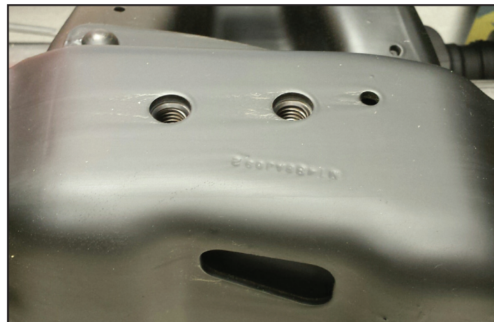
Upfit Body Frame ZW9 Attachment Provisions Figure 21
