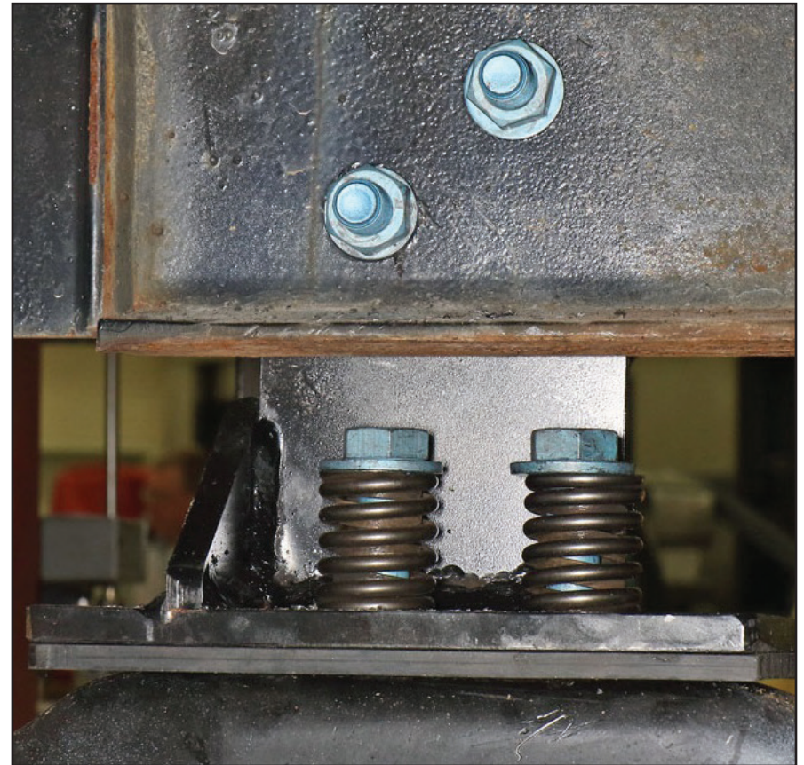
Combination U-Bolt, Shear Plate & Spring-loaded Forward Mount (ZW9)
