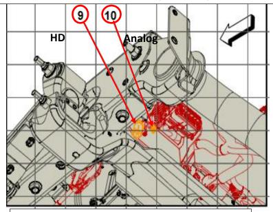
Mating (end gate) connector located rear of frame
