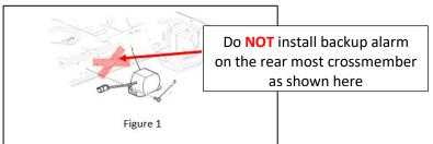
Installers must select an alternate location to mount the alarm assembly and the alarm be spliced into the reverse lamps circuit for power when vehicle is in reverse. Refer to page 51 of GM Upfitter Integration Electric Best Practices manual for recommendation on performing multiple wire splices (GM UI Electrical Best Practices)
