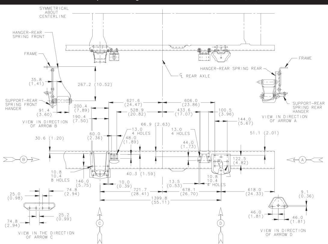
C 3500HD Rear Suspension Hanger Bracket Locations, Chassis Cab, 15,000 GVWR
