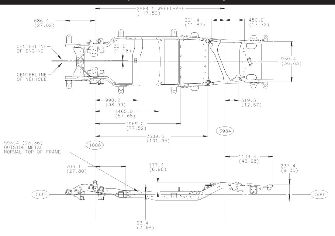
FRAME RAIL METAL THICKNESS 4 mm
