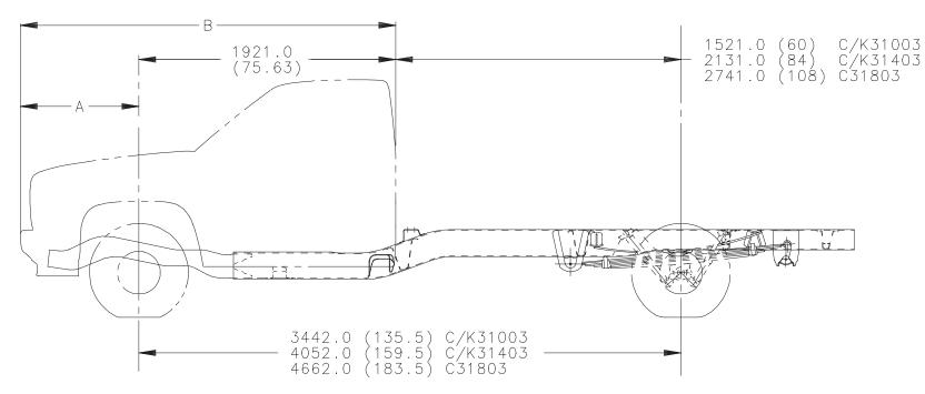
DIMENSIONS SHOWN ARE NOMINAL ESTIMATES BASED ON EVEN DISRIBUTION OF WEIGHT PRECENTAGES ALLOW FOR 3" CB (CAB/BODY CLEARANCE) DIM ADIM B10-12000 LB. GVW899.4<br/>(35.41)2820.3<br/>(111.03)15000 LB. GVW965.0<br/>(37.99)2886.0<br/>(113.62)
