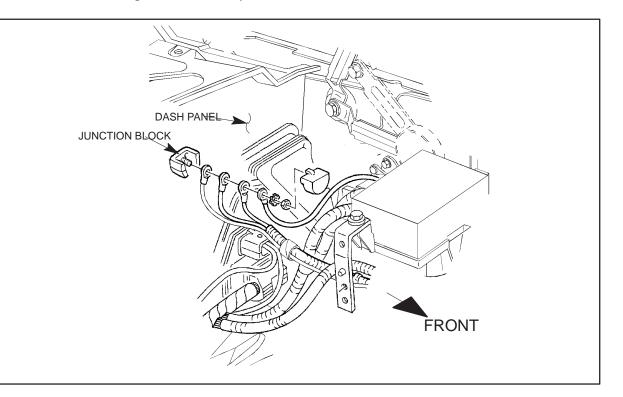
Also, for cab/chassis with the "YF2" option, heavy gauge ground straps have been provided between the engine, chassis and body sheet metal near the right rear of the engine for the purpose of providing a robust ground return path from the body or chassis to the battery. The body builder must ensure that the ground returns from their loads provide an adequate ground path into these straps such that voltage drops are minimized.
