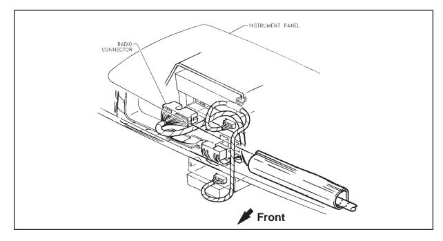
The radio may have to be removed from the instrument panel to gain access to the 20 pin connector.
