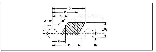
C.G. of vehicle in FMVSS unladen condition (Curb + 400 lbs.) must be inside shaded area – that is, it must be within the trapezoid formed by the coordinates A, B C, D, H<sub>1</sub> & H<sub>2</sub>, plus it must be to the rear of vertical line E and forward of vertical line F.
