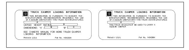
CONSUMER INFORMATION REGULATION 575.103 issued by the National Highway Traffic Safety Administration requires manufacturers of trucks capable of accommodating slide-in camper bodies to provide information concerning proper load and proper load distribution in truck-camper applications.
