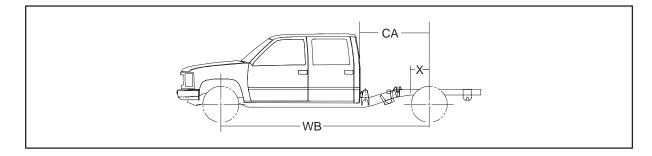
Body lengths, and percentage figures are found in the Body-Payload Weight Distribution Charts located in the model weight section for pickup and C/K chassis cabs. These charts represent all lengths that are possible to use. The shortest length in each case represents the smallest body that will reach the approximate end of the chassis frame at the maximum cut off. The longest length represents the largest body which can be used without placing the center of gravity behind the rear axle.
