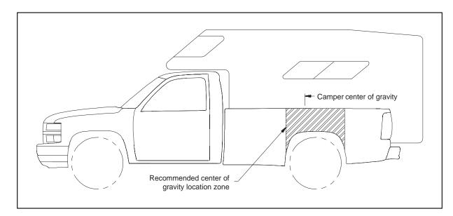
Any accessories or other equipment added to this vehicle, after final date of manufacture, must be weighed or have their weight determined, and the weight deducted from the prescribed cargo weight rating (CWR) of this vehicle. This may decrease the permissible longitudinal zone of the center of gravity for this vehicle.
