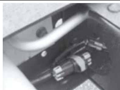
Back up Alarm connector located on LH rail of last cross member.
