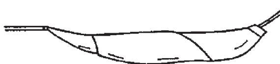
23. Additional tape can be applied to the wire if the wire does not belong in a conduit or another harness covering. Use a winding motion in order to cover the first piece of tape.
