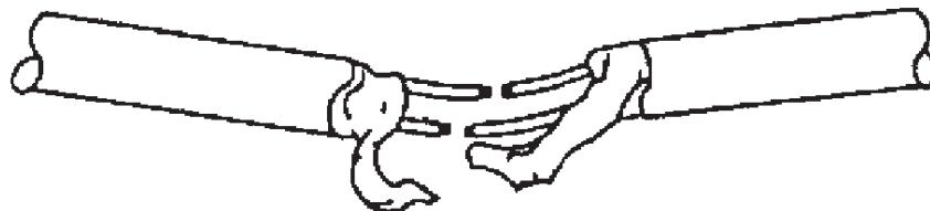
3. Prepare the splice. Untwist the conductors and follow the splicing instructions for copper wire. Staggering the splices by 65 mm (2.5 in) is recommended.
