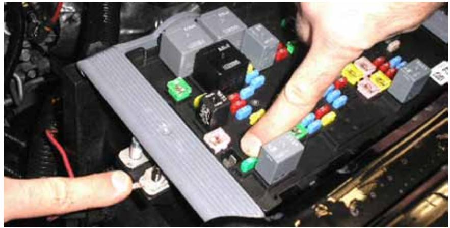
**Important:** Ensure that the ringlets are not interfering with the UBEC cover.
