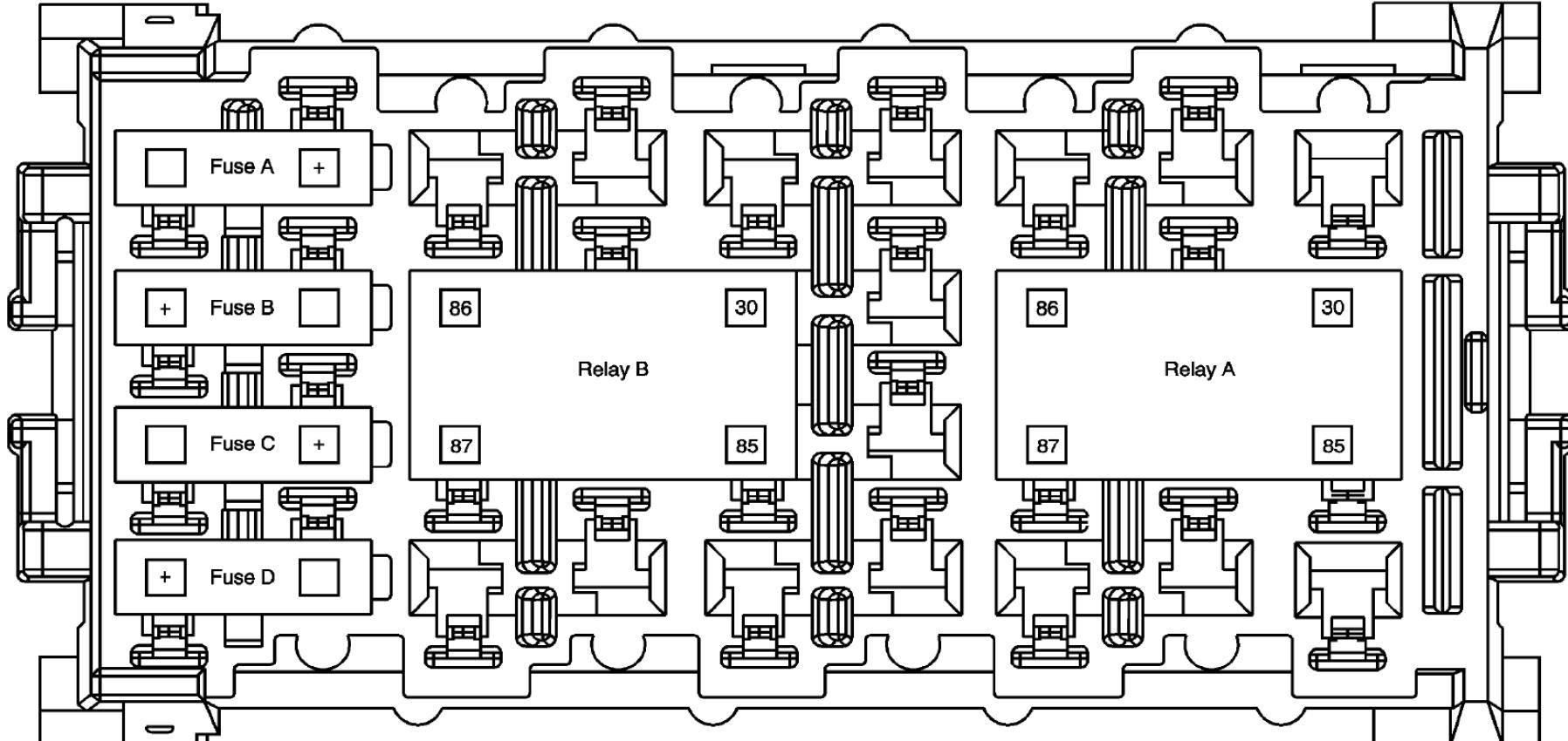
**Fuse Block - Mobile Radio, Device Usage (9L4)**
