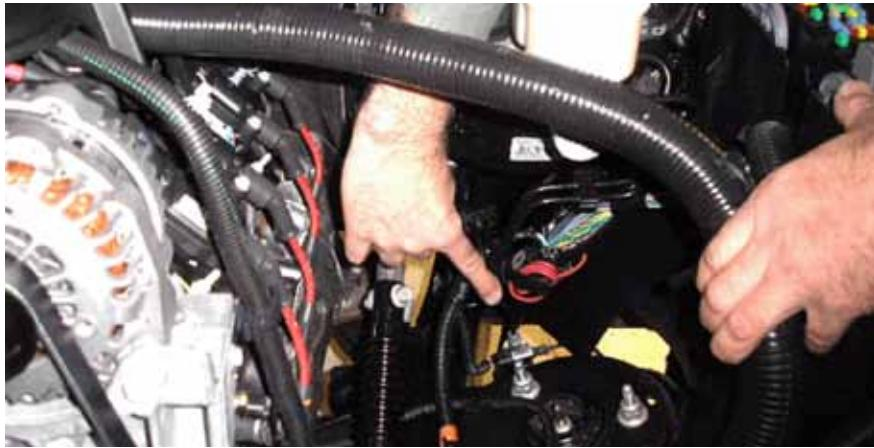
Circuit #742 for Auxiliary Power at the 7-way trailer connector is no longer connected by the GM Assembly Plant. If the customer desires auxiliary power at the trailer connector location (i.e. refrigeration, battery charger or interior light in the trailer), complete the following steps to connect circuit #742:
