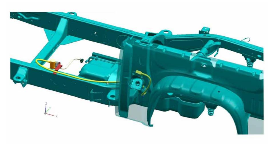
Note: Gas Models require Upfitter to permanantly mount Vapor Pressure Senser Unit in a sheltered environment. Sensor wire harness should also be secured properly. Harness and Sensor should be clear of moving and or heat generating chassis components.
