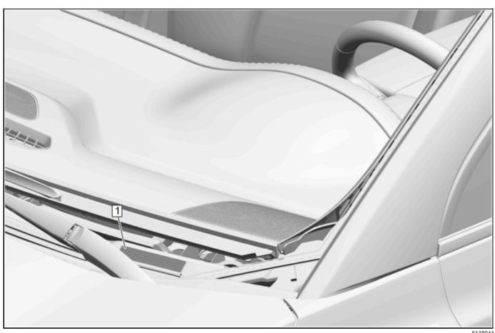
The VIN plate is the legal identifier of the vehicle. The VIN plate (1) is located on the upper left corner of the instrument panel (I/P) and can be seen through the windshield from the outside of the vehicle:
