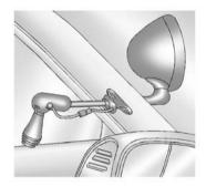
A Unity Series 330, high intensity, 100 watt halogen (H3 bulb) 15 cm (six inch) spotlamp is mounted in the left windshield pillar. The lamp is protected by a 15 amp fuse located in the instrument panel Intermediate Electrical Center-Left. See the service manual for lamp replacement procedures.
