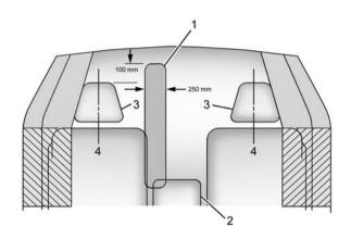
Optional Driver Seatback Front Center Airbag Deployment Zone (RPO AYQ and D07) – View from Rear Cargo Area
