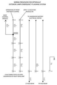
Forward Lamp Harness In-Line Connector for use with Headlamps Flasher Module, Option 6J7
