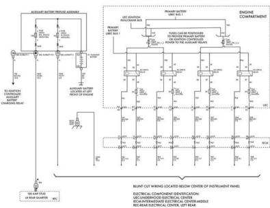
Wiring Provisions – 12-Volt Battery Power
