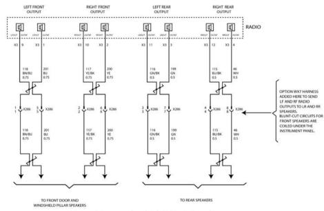
Wiring Diagram for SEO WX7 Inline Connector
