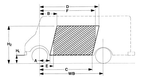
C/G of vehicle in CMVSS or FMVSS unladen condition [Curb + 181.4 kg. (400 lb) for vehicles less than or equal to 4536 kg (10,000 lbs) GVWR or Curb + 226.8 kg (500 lbs) for vehicles greater than 4536 kg (10,000 lbs) GVWR] must be inside shaded area – that is, the C/G must be within the trapezoid formed by the coordinates A, B, C, D, H1, & H2, plus the C/G must be to the rear of vertical line E and forward of vertical line F.
