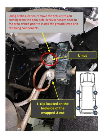
Clean the area of the exhaust hanger hook as noted in the picture above. Using a U-nut (P/N 9431352) and a J-Clip (P/N 15149848) Install a ground strap as shown from the body/frame exhaust hanger hook to the muffler/exhaust system hanger hook.
