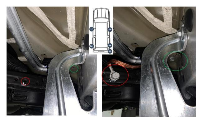
Fasten 1 provided ground strap from left front frame body mount bracket using an M8x1.25 bolt/screw and an M8 nut using the provided hole in the back wall of the bracket (A) (position the ring terminal neck as shown) to a provided hole (B) on the backside of the body cross member using a M8x1.25 bolt/screw (position the ring terminals as shown).
