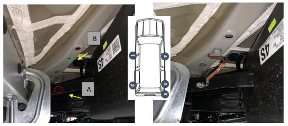
Fasten 1 provided ground strap from left front frame body mount bracket using an M8x1.25 bolt/screw and an M8 nut using the provided hole in the back wall of the bracket (A) (position the ring terminal neck as shown) to a provided hole (B) on the backside of the body cross member using a M8x1.25 bolt/screw (position the ring terminals as shown).
