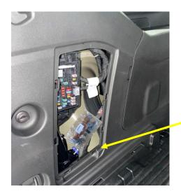
Kit is shipped in the rear electrical center behind the close out cover
